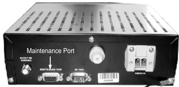
Figure 46: Maintenance Port on MCU
