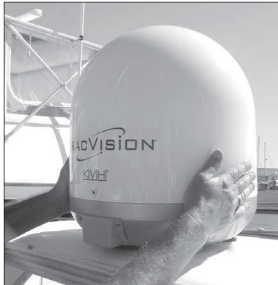
Figure 11: Removing the Radome
