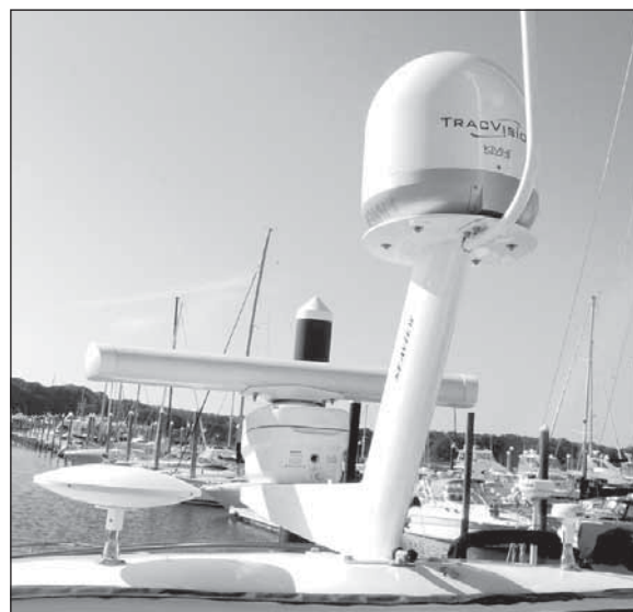
Figure 28: Radome Labels Facing Fore and Aft
