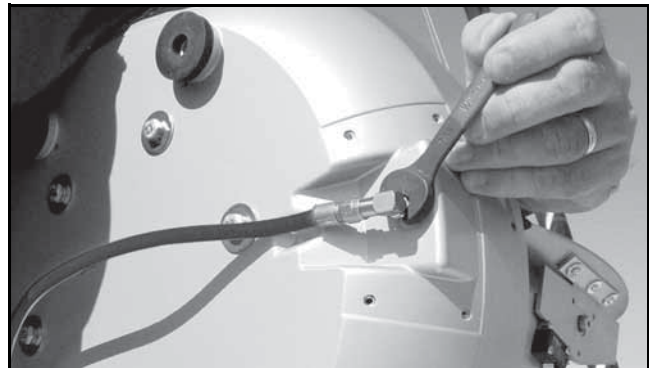
Figure 10: Protecting the Cable Connection
