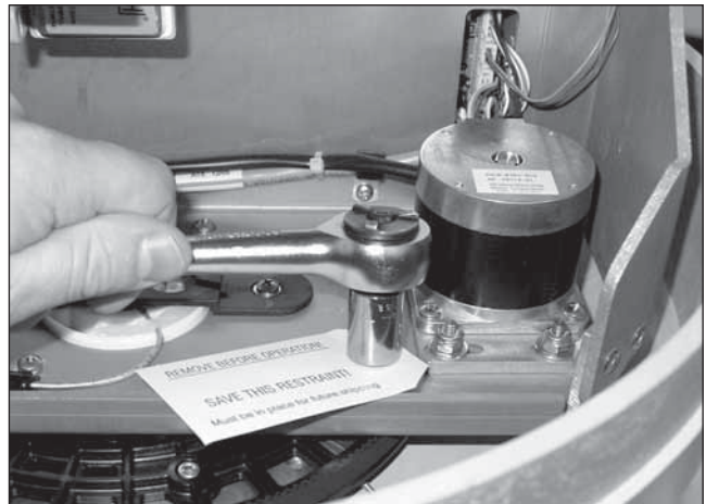
Figure 12: Removing the Shipping Restraint
